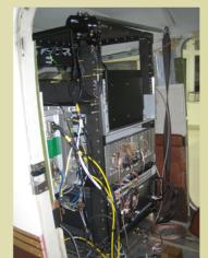
Left: Vibration isolated 19" rack provides quick mounting of standard rack mount equipment. ATR chassis and odd shaped research payloads are easily accommodated.
